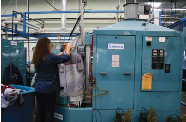
An employee places a work shirt on a shirt press. POS still presses all its work shirts; work pants are processed through a tunnel finisher.
