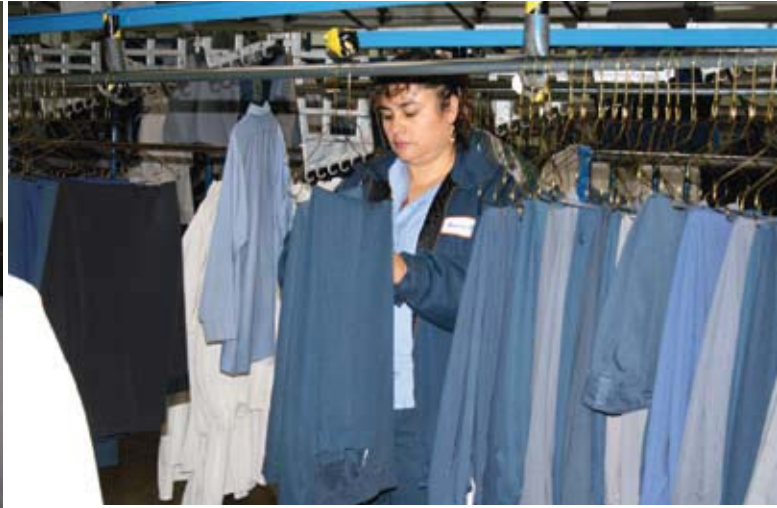
An employee places work pants on hangers for movement to the overhead rail system that takes them to the tunnel finisher.
