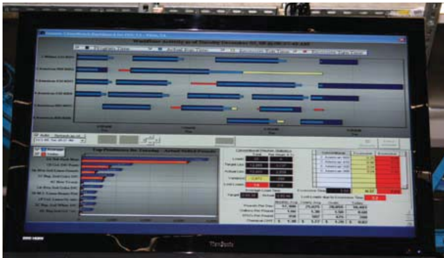
This Ultrax overhead screen from Dober tells POS/Vista employees in the wash aisle how they're progressing in terms of the productivity of employees and machines. The plant is expected to upgrade its monitoring program this year to Dober's Spindle system.
