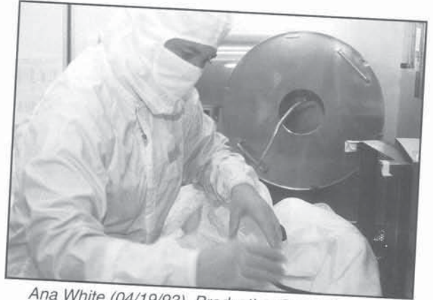
Ana White (04/19/93), Production Supervisor and Back-up QA Technician, tests a garment for ESD.
