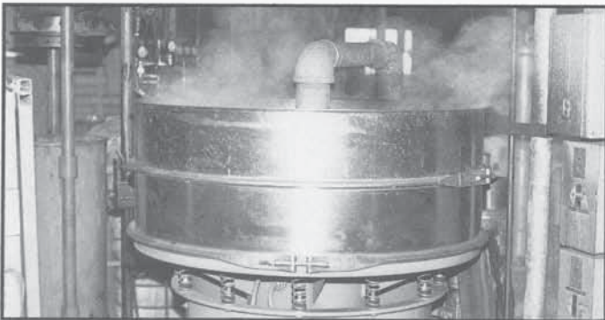
This machine uses a shaking motion to separate water from solid waste. The water is then recycled into the sewer system and the solid waste is put into special storage containers for proper disposal.
