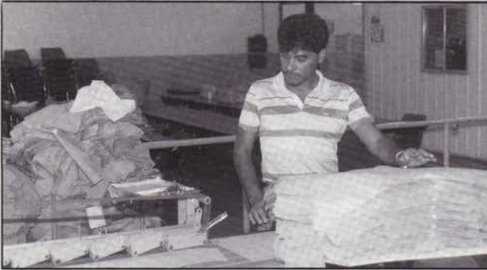
Vicente Rodriguez uses a Hem Front Machine to prepare the front of the garments.
