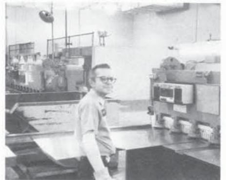
Steelcase machine operator Wayne Troemper runs the shear, which cuts sheets of steel down to required sizes.
