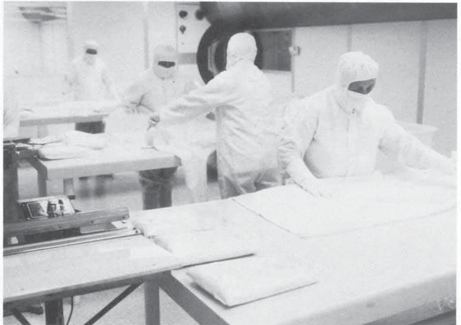
Employees who fold, package, and air tight seal inside the clean room are gowned to protect the product.
