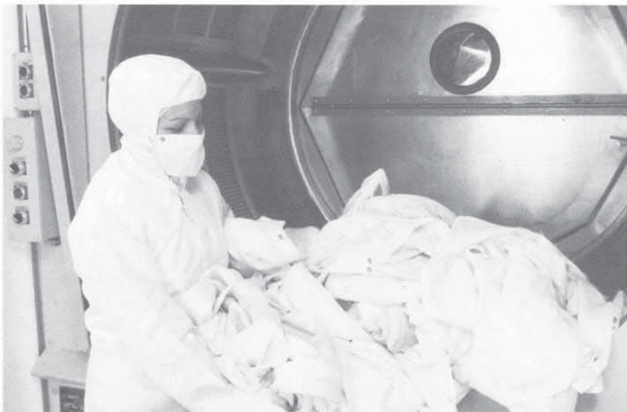
Employee unloading barrier air dryer with HEPA filtered air supply inside the clean room where gowning is necessary and no solvent or moisture is allowed.
