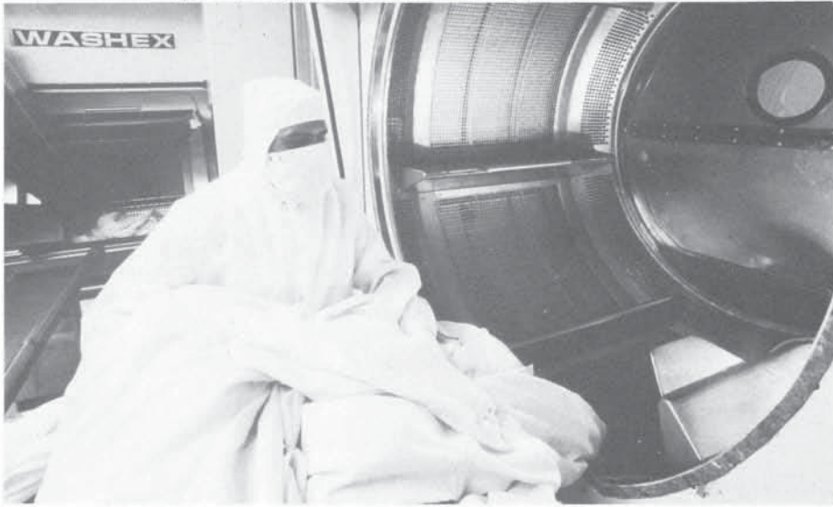
Clean laundry is loaded into the dryer inside the clean room, where proper clean room apparel is worn.
