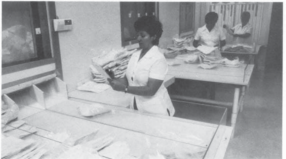
Garment packages leave the clean room via special designed positive pressure pass through chutes to the distribution area.
