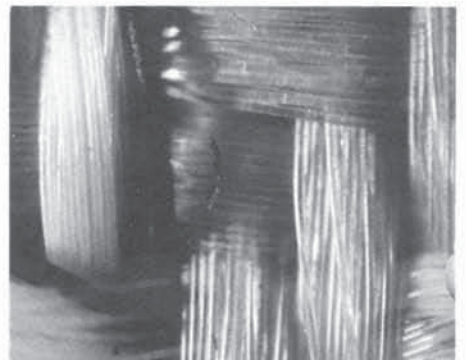
Here you can see how they weave carbon nylon fiber to create the grid effect.
