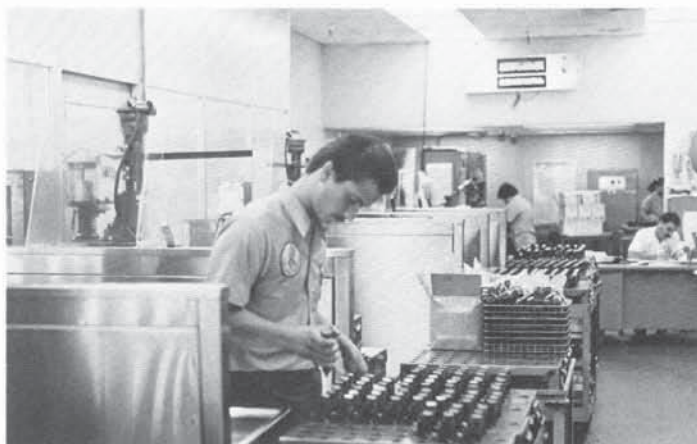
Detroit Diesel fuel injectors are re-manufactured in the Production Rebuilding Division.
