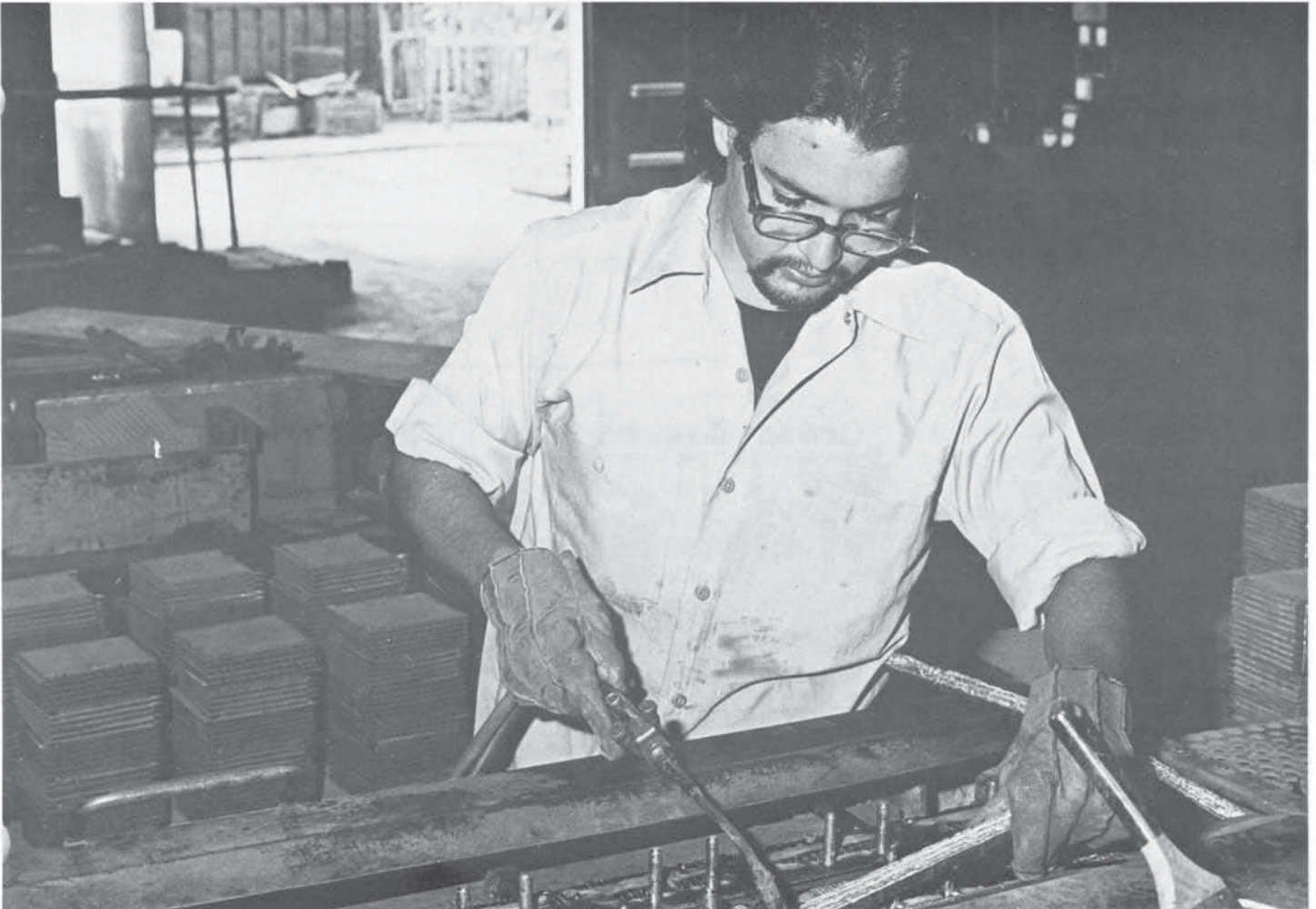
Employee solders lead posts onto newly constructed batteries. Uniforms play a key role in the company's industrial health program.
