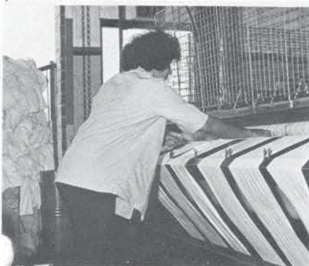
Emma Quintana feeds automatic towels through the eight-roll ironer. Here, too, are processed hand towels, sheets and pillow cases, smocks and aprons.
