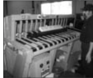
Mat Roller - Logo mats are rolled and are identified by an RF chip. The mat roller is equipped with an RF chip reader to identify the route, customer, and delivery day.
