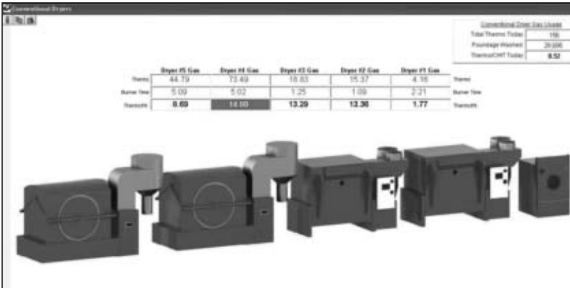
Dryer View is a 3-D view of each facility's dryers. The image shows natural gas total usage, burner time, average consumption for each dryer and a conventional dryer gas usage chart. There are also red and yellow parameters set for individual dryers to help recognize potential problems.
