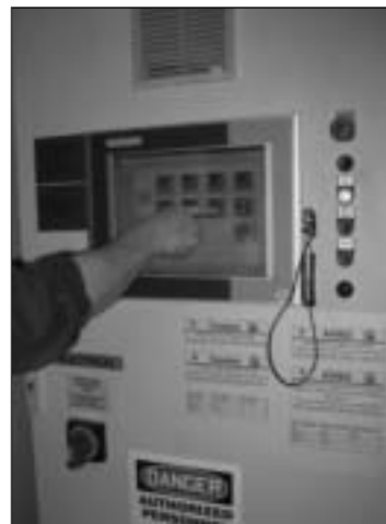
Microprocessor – Jensen dryers are controlled by a microprocessor which control temperature by infrared sensors.
