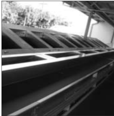
Soil Sorting Bins – Merchandise is sorted by type and weight to fill slings for wash loads.
