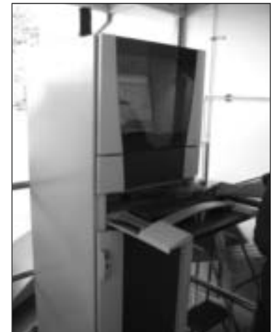
Computer Terminals – This terminal control soil sorting bins and overhead rail storage system.
